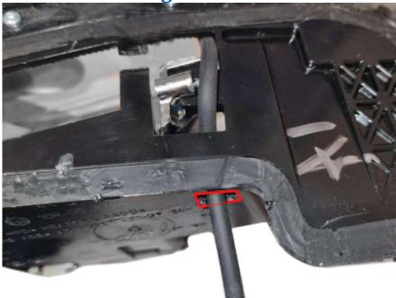
Avoid pulling on the wires on the emitter.
